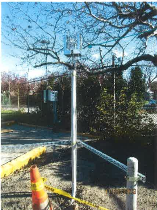
Photograph 2 – Solar powered wet sensor electronic housing
